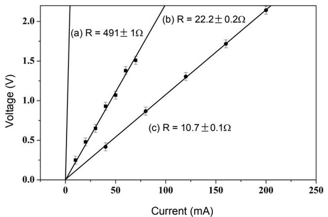
Fig. 4. Typical nanowire resistance curves. (a) A wire on top of contact pads before reflow with a high contact resistance, (b) a wire on top of contact pads after reflow with a small contact resistance, and (c) a wire underneath the contact pads with minimal contact resistance.
