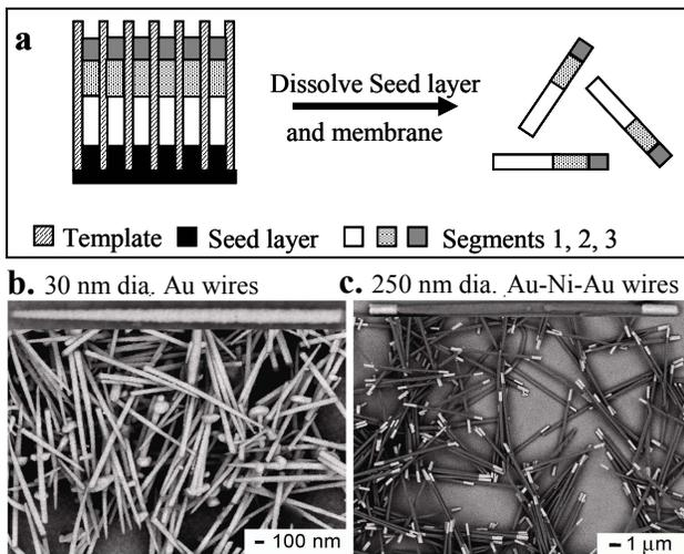
Fig. 1. (a) Schematic diagram of the strategy used to fabricate nanowires using electrodeposition in a nanoporous template. SEM images of (b) 30 nm diameter gold wires, and (c) 200 nm diameter Au-Ni-Au wires. (The back scatter contrast is brightest for metals with higher atomic numbers, Au appears brighter than Ni).
