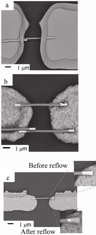
Fig. 3. (a) SEM image of contact pads aligned over the ends of a nanowire using photolithographic patterning. SEM image of (b) two wires, and (c) a single wire deposited on top of pre-fabricated contact pads using magnetic assembly.
