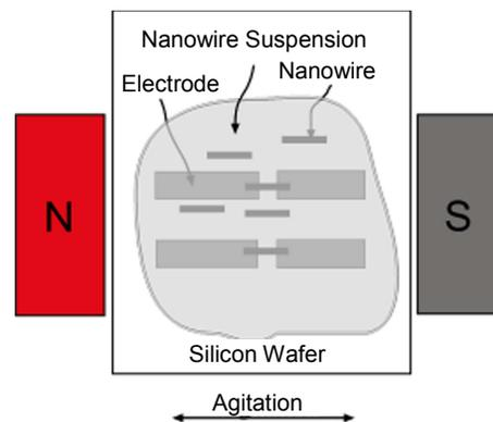
Fig. 2. Schematic diagram of directed assembly using magnetic fields.
