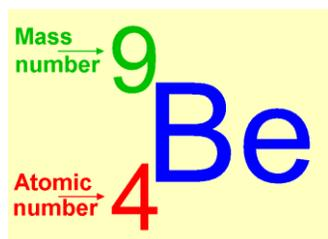
**Figure 1–5** Standard format for reporting atomic number and mass number. This isotope of beryllium has four protons and five neutrons.
