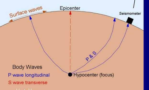
The arrival of earthquakes waves is recorded by a seismograph. The amplitude of the P-wave displacement is used to determine the Richter magnitude.
