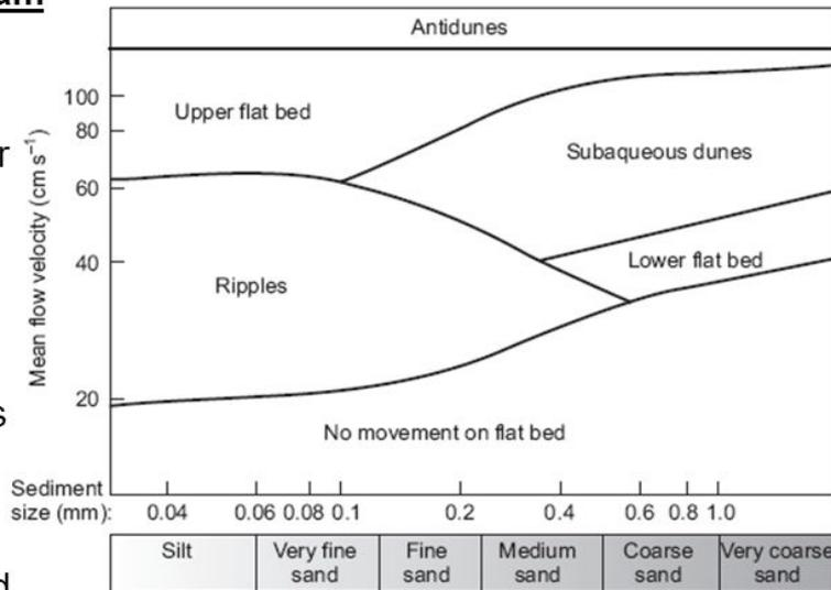
A bedform stability diagram which shows how the type of bedform that is stable varies with both the grain size of the sediment and the velocity of the flow.
