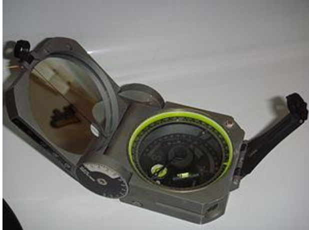
Figure 2. Brunton compass showing bulls eye and bubble levels.
