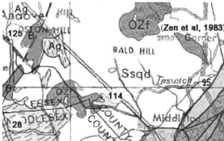
Figure 3. The bedrock geology in the vicinity of the Jenkins Quarry consists of four formations within the Nashoba Terrane. These include; the Andover Granite, Sharpners Pond diorite, Boxford Formation and Fish Brook Gneiss. The Andover Granite contains numerous small outliers of the Boxford formation. Many of these are associated with faulting and/or pegmatites. The Sharpners Pond diorite has intruded the Boxford Formation along old structural features.
