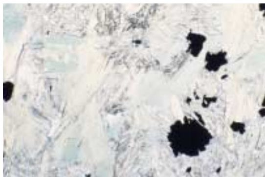
Figure 4a. Jenkins blue soapstone. Chlorite, clinoamphibole (actinolite?), talc, and magnetite. Field of view, 2 mm. Plane light.
