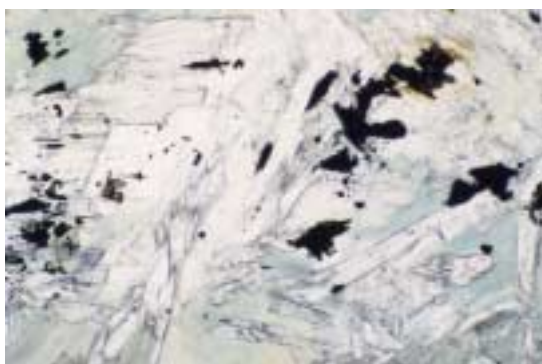
Figure 5a. Massive Green Soapstone. Chlorite, talc, clinoamphibole, and magnetite. Field of view, 2 mm. Plane light.
