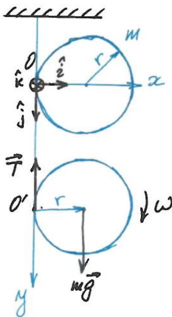
Suppose that initially the disc has a point O in contact with a string and that after time t the disc has rotated through angle  $\theta$ .
