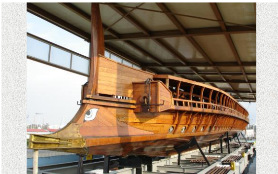
Olympias, a reconstruction of an ancient Athenian trireme sea trials in 1987, 1990, 1992 and 1994 The bronze bow ram weighed 200 kg. The ship was built from Oregon pine and Virginia oak
