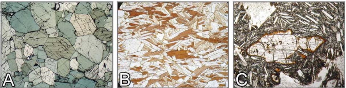
Figure 3.1-5: Subhedral grain shape A: Amphibolite; B: Biotite-muscovite schist; C: Olivine in basalt
