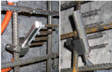
(c) Concrete corrosion and Humidity sensors
