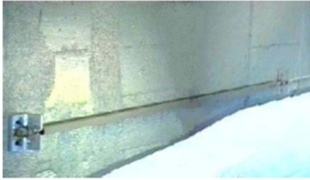
(a) Long-gauge SOFO fiber optic sensor
