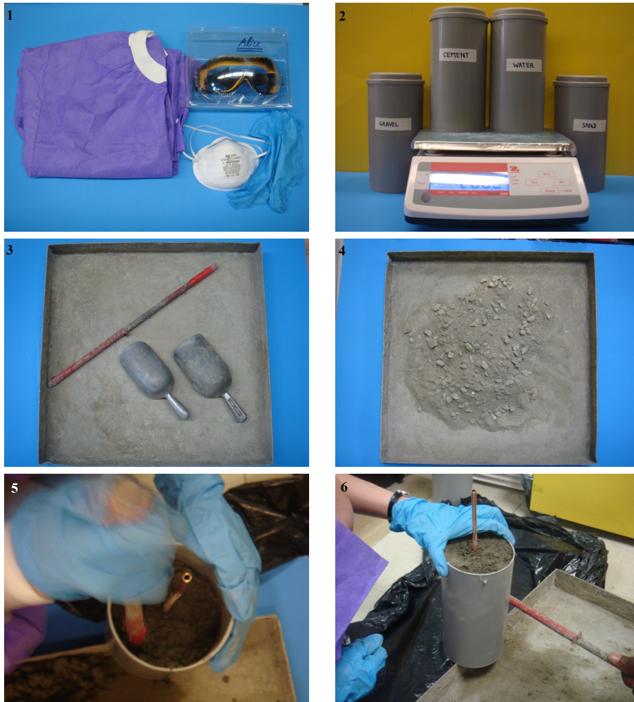
Figure 3-2: Casting concrete procedure
