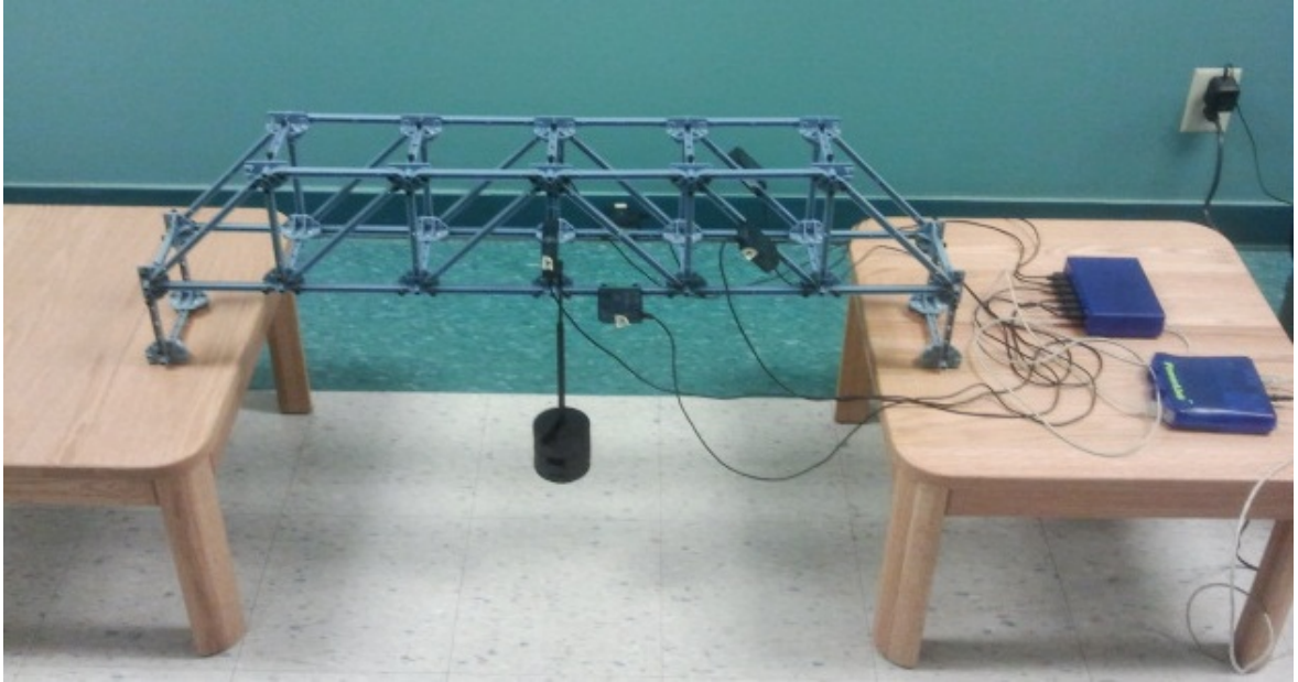
Figure 4-9: Experimental loaded intact truss bridge-Member 5
