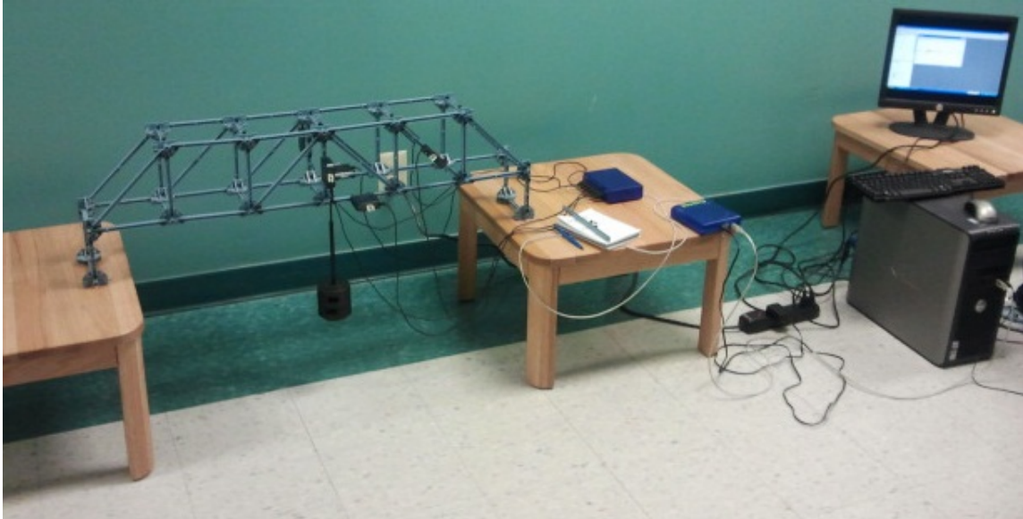
Figure 4-11: Experimental loaded damage truss bridge
