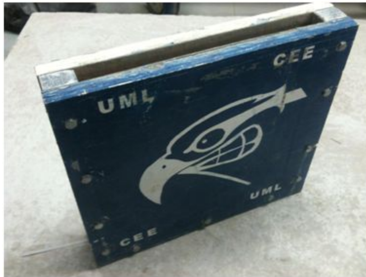
Figure 3-8: The inner surfaces of molds have been covered with plexiglass
