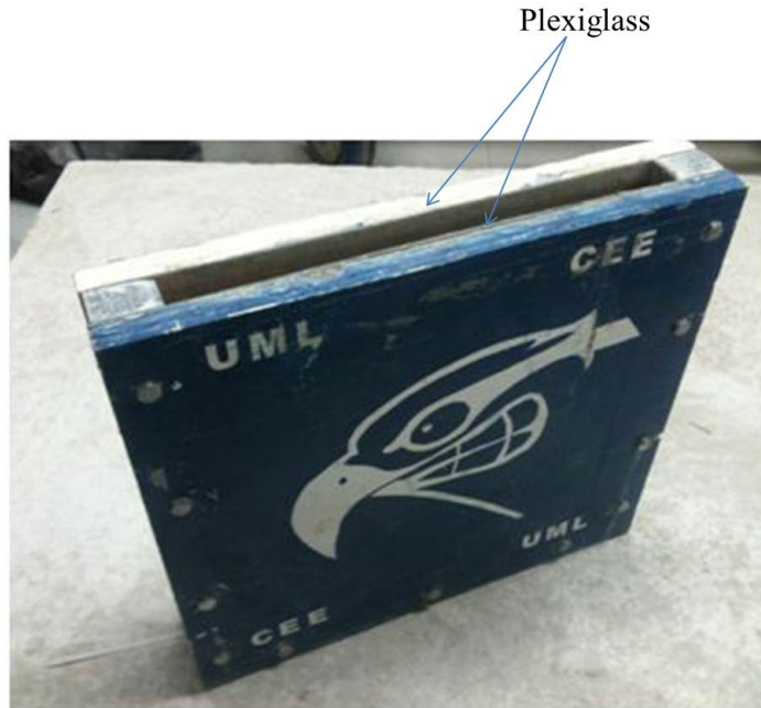
Figure 3-2: The mold with inner plexiglass surface
