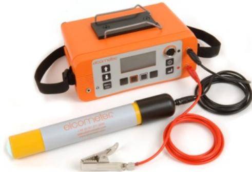
Figure 3.1: Half-Cell Sensor
