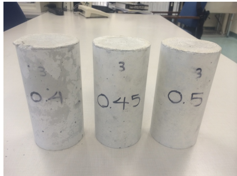
Figure : Oven Dried Concrete (Side View).
