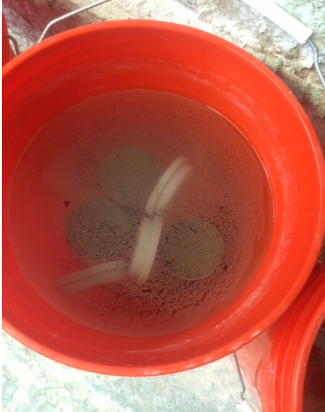
Figure : Curing Process.
