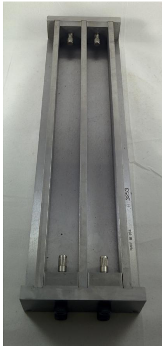
Figure 3-2: Molds used for mortar bars.
