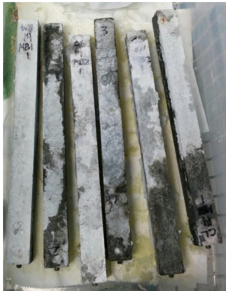
Figure A-2: 14-day mortar bars (left to right - AG3 MB1 , AG3 MB2 , AG2 MB2 , AG2 MB1 , AG1 MB2 , AG1 MB1 ).
