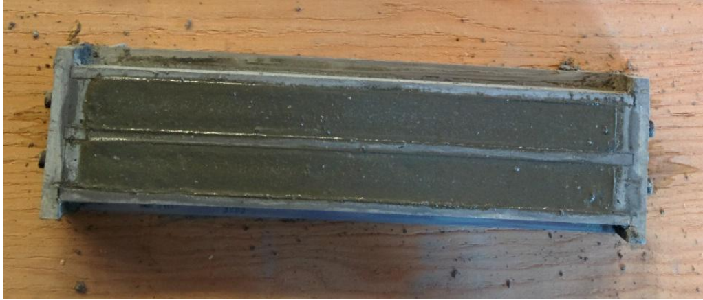
Figure 3-3: Cement mortar mix distributed into mold.
