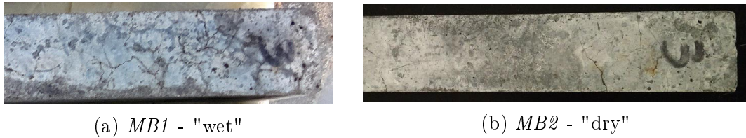
Figure 4-3: 28-day mortar bars made from AG2 aggregate.
