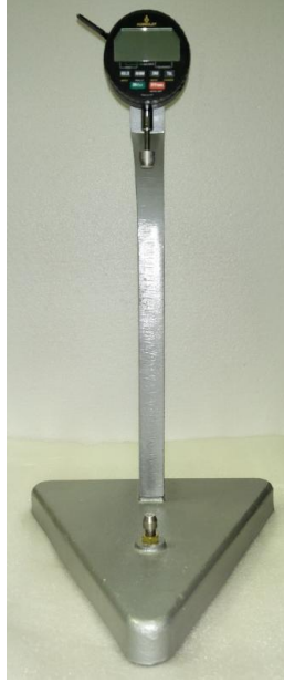
Figure 3-5: Length comparator for measurement of length expansion percentage.
