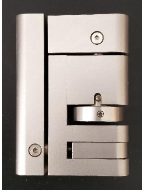
Figure 3-13: Shorting kit for calibration for dielectric measurement.
