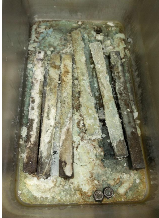
Figure 3-16: ASR gels leached out of mortar bars.
