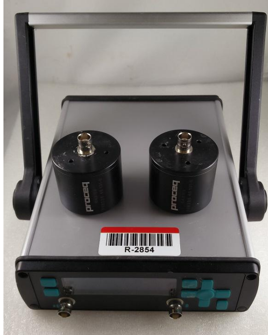
Figure 3-10: Proceq Pundit ® Lab with 54 kHz frequency transducer pair.
