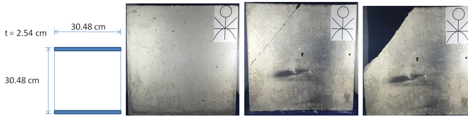
Figure 3-4: 30.48 cm square panels 2.54 cm thick; (left to right) PN01, PND01, PND02
