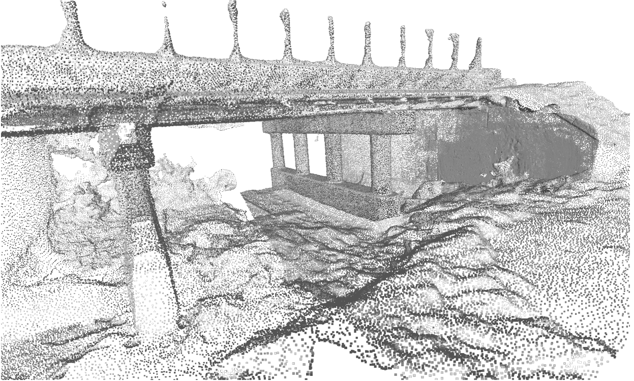
Figure 5-2: Plain Street bridge, Lowell MA. visual inspection model
