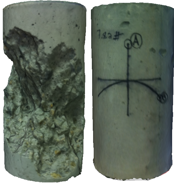
Figure 4-1: CN01.1 (left) shattered specimen & CN04 (right) intact specimen
