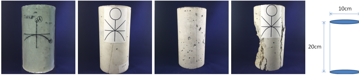
Figure 3-3: 10 cm x 20 cm cylinders; (left to right) CN02, CN03, CND01, CN04
