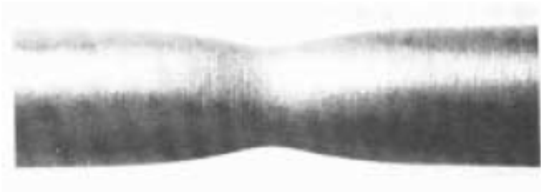
Necking in a tensile specimen
