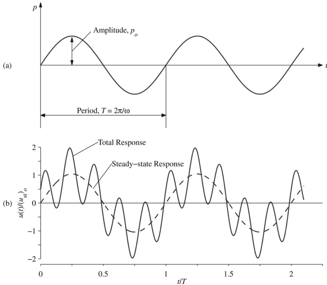
Figure 2: Harmonic force and the displacement response of an undamped SDOF system ;  $\frac{\omega}{\omega_n} = 0.2$ ,  $u_0 = \frac{p_0}{2k}$
