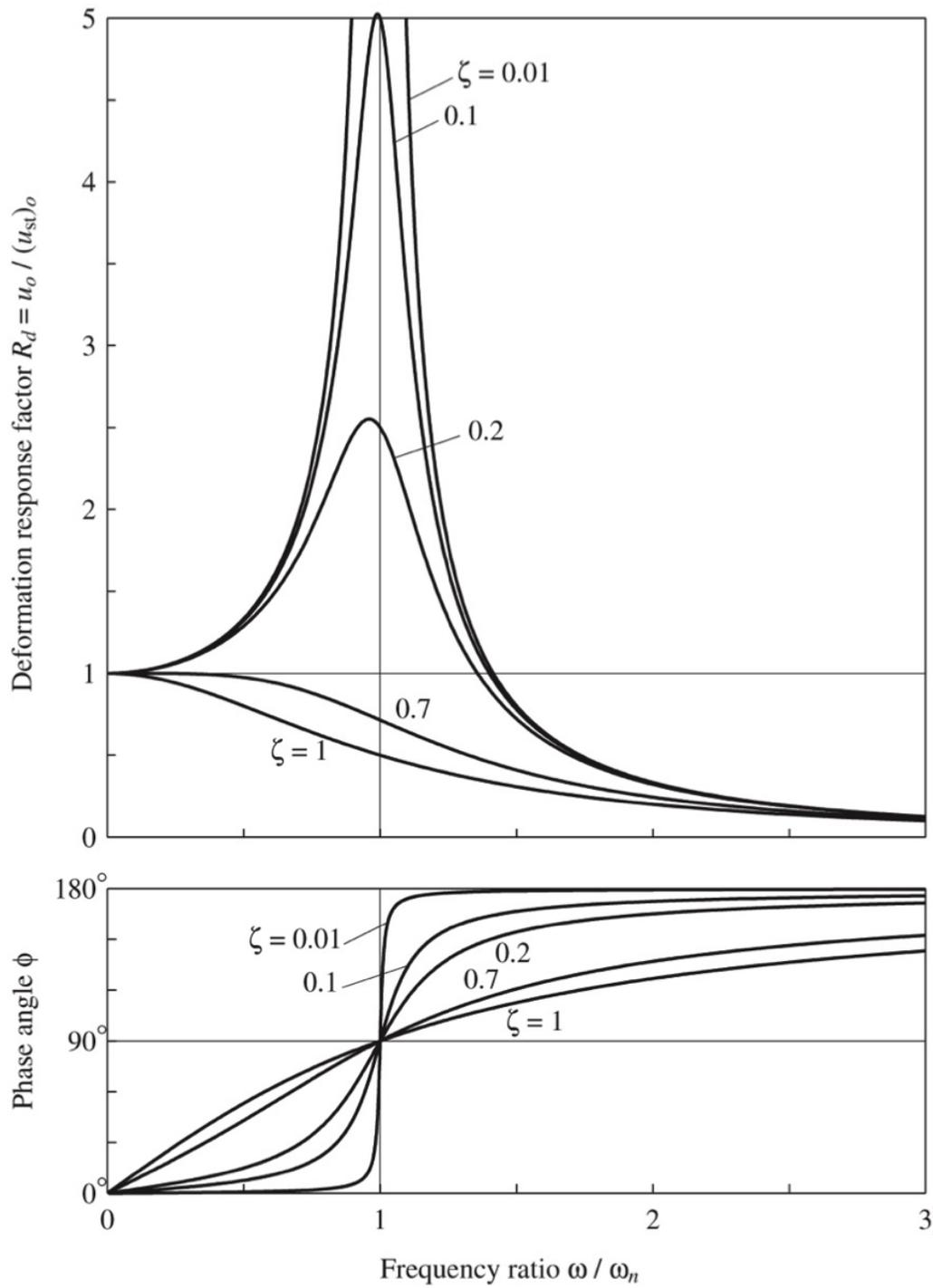
Figure 5: Deformation response factor and phase angle for a damped system excited by harmonic force
