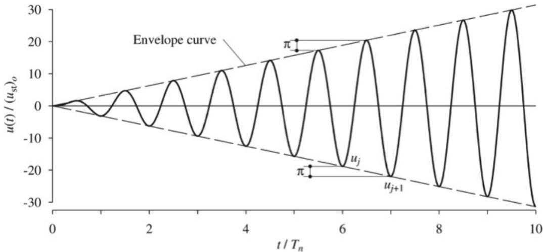
Figure 4: Displacement response ratio of an undamped SDOF system;  $\frac{\omega}{\omega_n} = 1$ ,  $\xi = 0$ ,  $u_0 = \dot{u}_0 = 0$ ,
