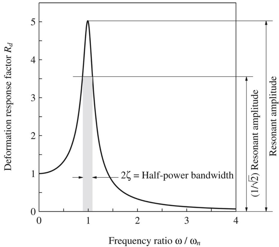
Figure 7: Definition of half-power bandwidth
