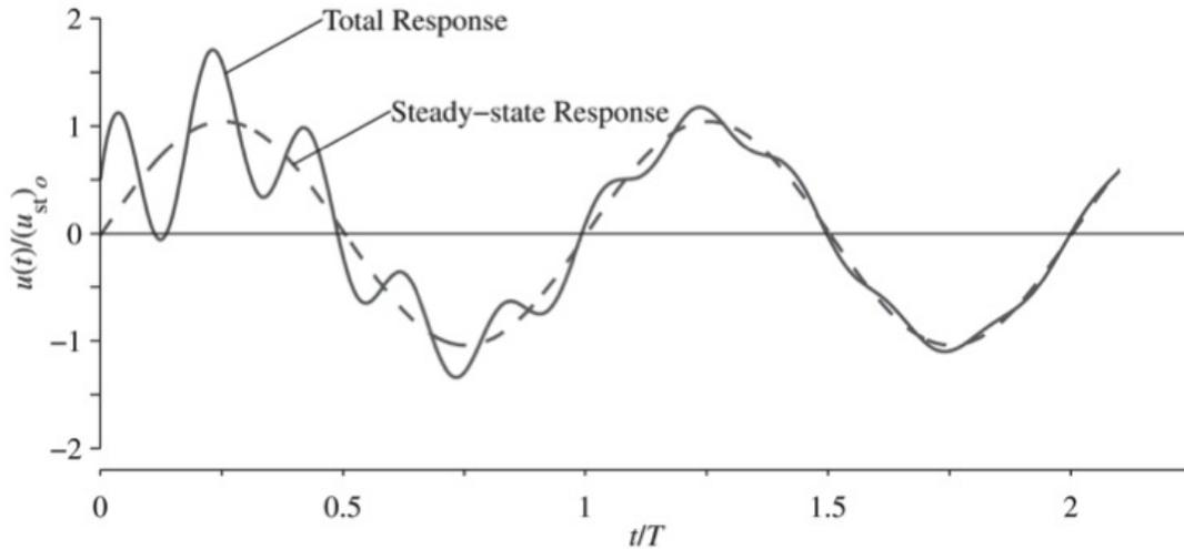
Figure 3: Displacement response of an undercritically-damped SDOF system;  $\frac{\omega}{\omega_n} = 0.2$ ,  $\xi = 0.05$ ,  $u_0 = \frac{p_0}{2k}$
