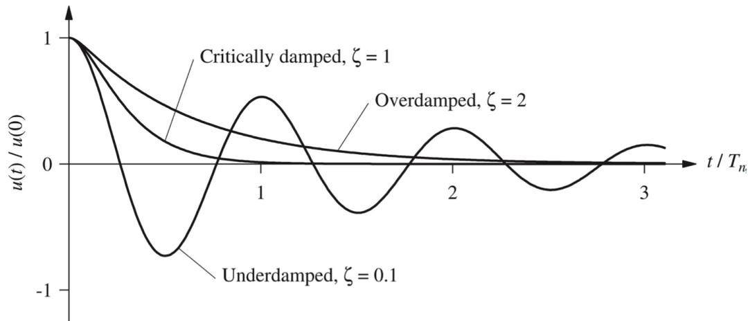
Figure 1: Free vibration displacement response ratio of SDOF systems
