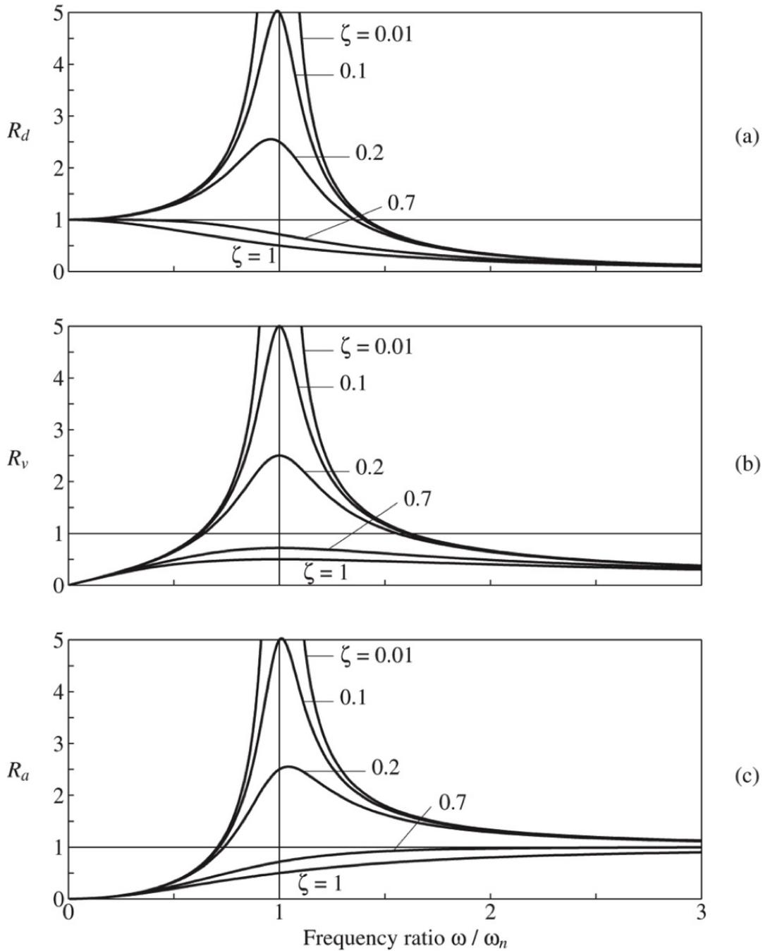
Figure 6: Deformation, velocity, and acceleration response factors for a damped system excited by harmonic force
