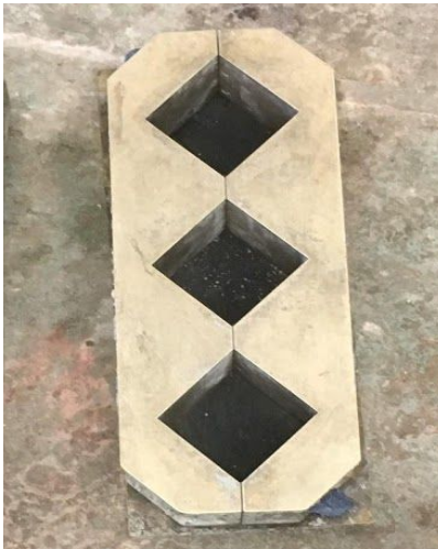
Figure 1. Steel Mold - 2 cubic inch
