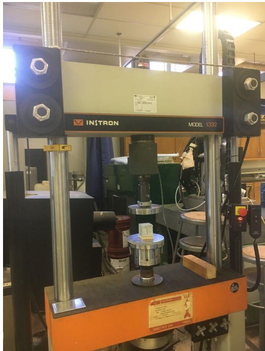
Figure 8. Compressive Strength Testing Apparatus used for Experiment 2, Instron Model 1332
