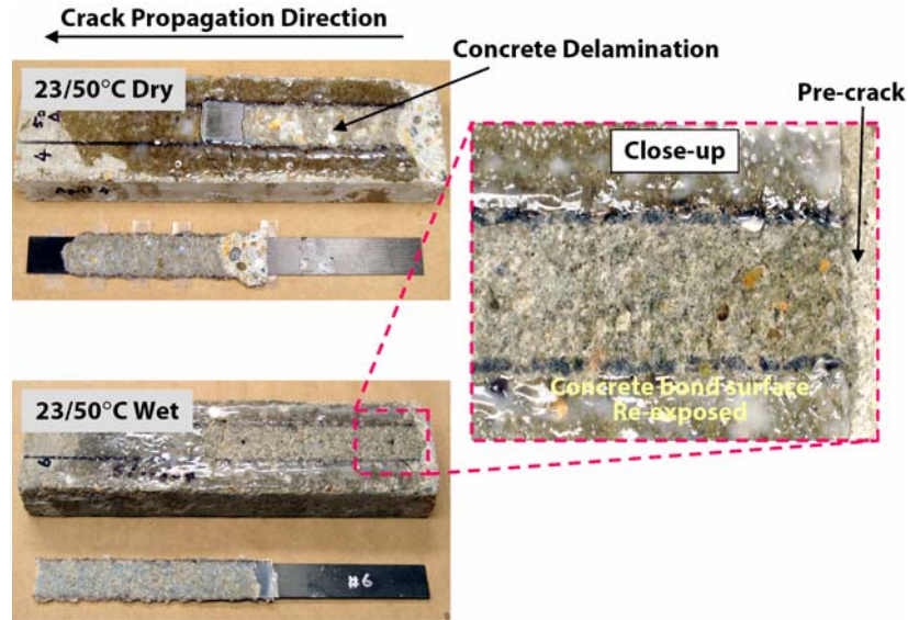
Figure 5 Shear debonding modes (Au and Büyüköztürk, 2006a).
