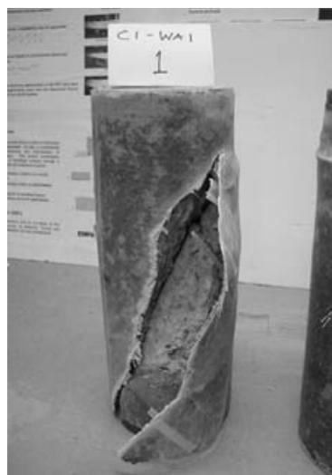
Fig. 2 Global shear cracking
