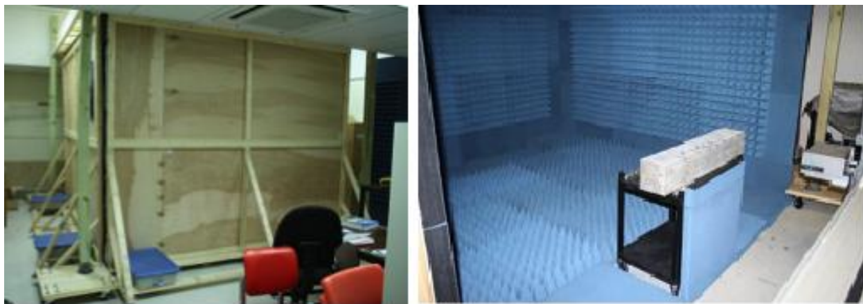
Figure 4. Custom-built anechoic chamber, 1 GHz-18 GHz; (left) exterior of the chamber, (right) interior of the chamber with a reinforced concrete beam specimen (CEE, UML)
