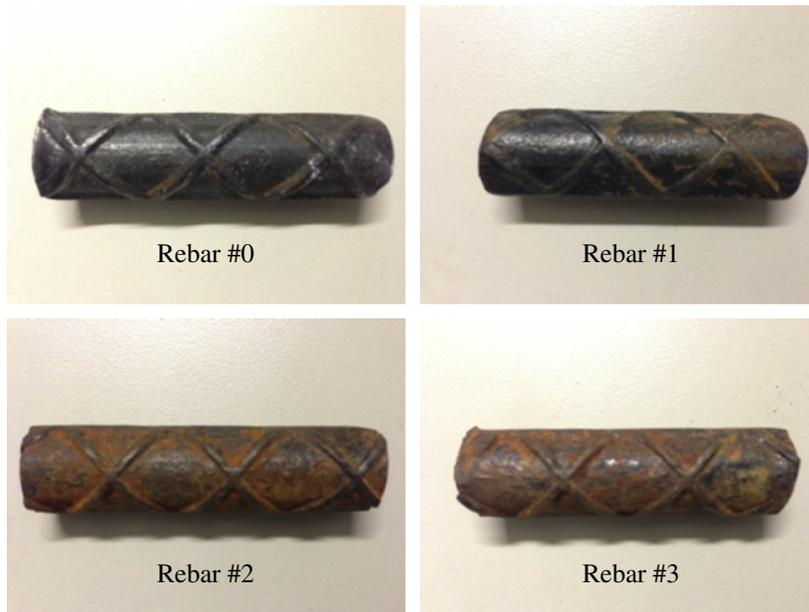
Fig. 6. The photo assessment of the samples with different corrosion rate.
