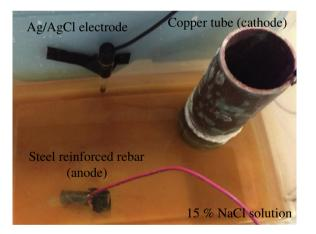
Fig. 3. Photo of the corrosion reactor setup.
