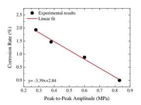
Fig. 9. Corrosion rate trendline estimates from peak-to-peak amplitude.
