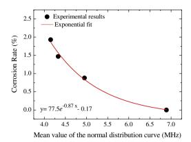
Fig. 13. Corrosion rate trendline estimates from mean values of the normal distribution curves.
