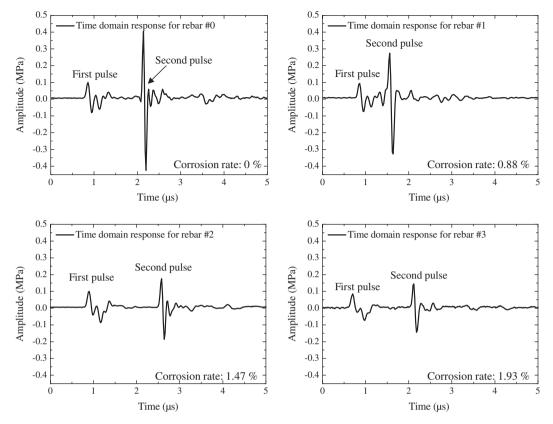
Fig. 8. Time domain responses for rebar samples.
