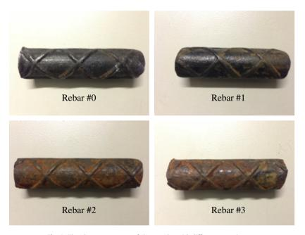
Fig. 6. The photo assessment of the samples with different corrosion rate.
