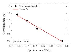
Fig. 11. Corrosion rate trendline estimates from spectrum area.
