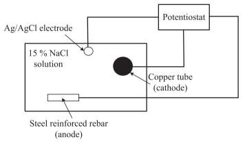
Fig. 2. Schematic diagram of the corrosion reactor setup.
