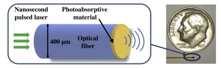
Fig. 1. Structure of the fiber optic ultrasound generator.
