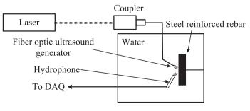
Fig. 4. Schematic diagram of the nondestructive corrosion detection setup.
