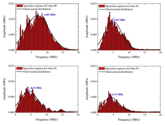
Fig. 12. Spectrum responses and the fitted normal distribution curves for rebar samples.
