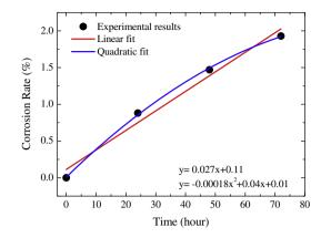
Fig. 7. Corrosion rate trendline estimates from reaction time.
