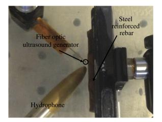
Fig. 5. The photo of the nondestructive corrosion detection setup.
