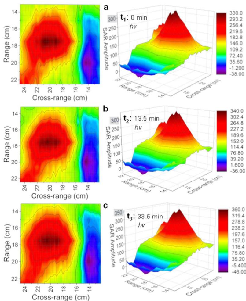
**Fig. 7** Distant monostatic reflective SAR images of a triangular glass plate partially coated with **2**. a) Image profile with no light. b) After 15 min. c) After 30 min of LED-white light illumination. It shows signal amplification going from  $t_1$  to  $t_3$  at 0.5–4.0 GHz.
