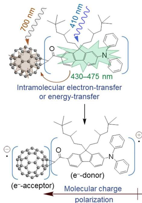
**Fig. 1** Conjugation structure of  $C_{60}$ (>DPAF- $C_9$ ) **1** at the keto conjunction, where the keto-enol isomerization resonance<sup>31</sup> is omitted, showing optical absorption wavelength ranges of the donor and acceptor moieties and the photoinduced intramolecular  $e^-$ -transfer in a close distance of only few Å leading to the formation of a molecularly polarized charge-separated state.
