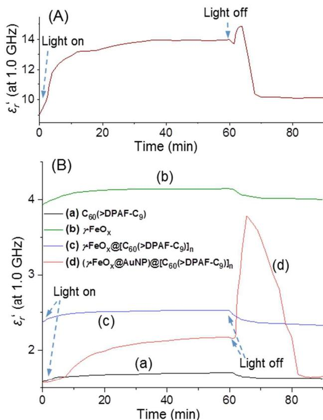
**Fig. 5** Large photoswitchable amplification of relative dielectric constant ( $\epsilon_r'$ ) of trilayered samples of **2** at the light-off state. Time-dependent  $\epsilon_r'$  profiles of five samples at 1.0 GHz; (A) ( $\gamma$ - $FeO_x@AuNP$ )-PDMS and (B) various samples as indicated.
