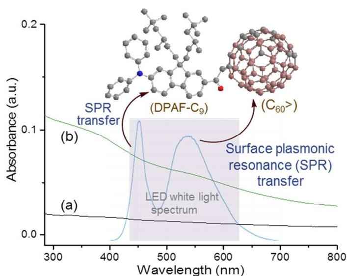
**Fig. 4** UV-vis absorption of (a)  $\gamma$ -FeO<sub>x</sub> NPs and (b) core-shell  $\gamma$ -FeO<sub>x</sub>@AuNPs with their broad absorption bands overlapping with two emission bands of white LED light used. SPR energy generated from either 450-nm or 540-nm band irradiation is capable of inducing the excitation of DPAF-C<sub>9</sub> or C<sub>60</sub>> cage moiety, respectively.
