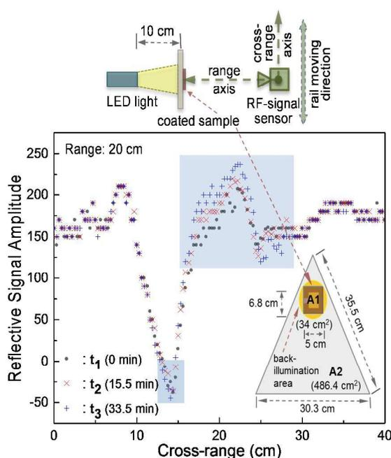
**Fig. 8** Cross-range reflective signal amplitude of a 2-coated triangular glass plate (inset, core-shell sample-coated A1 area with uncoated A2 area) with or without LED-white back-light illumination;  $t_1$ , No light;  $t_2$ , 15-min;  $t_3$ , 30-min irradiation. Experimental setup configuration is shown on the top.
