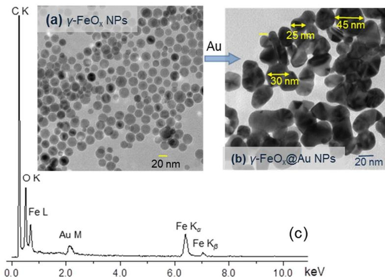
**Fig. 3** Micrographic images of (a)  $\gamma$ -FeO<sub>x</sub> and (b)  $\gamma$ -FeO<sub>x</sub>@AuNP NPs, used for the measurement. (c) Energy dispersive spectrum (EDS) of  $\gamma$ -FeO<sub>x</sub>@AuNP showing the composition where the carbon arises from the carbon tape used for the sample preparation and the oxygen is from both the sample and the environment. The result indicates a molar ratio of Fe: Au as roughly 13:1.
