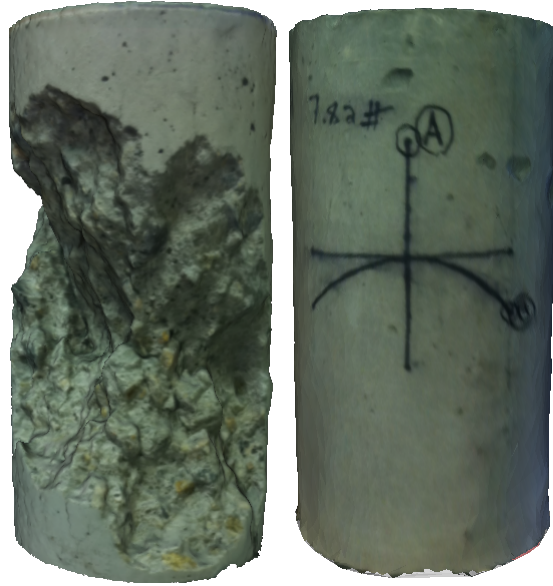
Figure 2. Model 1 (left) shattered Specimen & Model 2 (right) intact specimen
