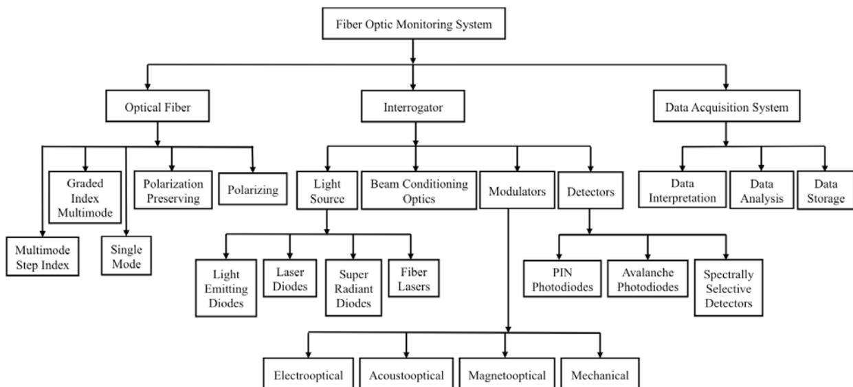
Figure 1. Overview of fiber optic monitoring systems
