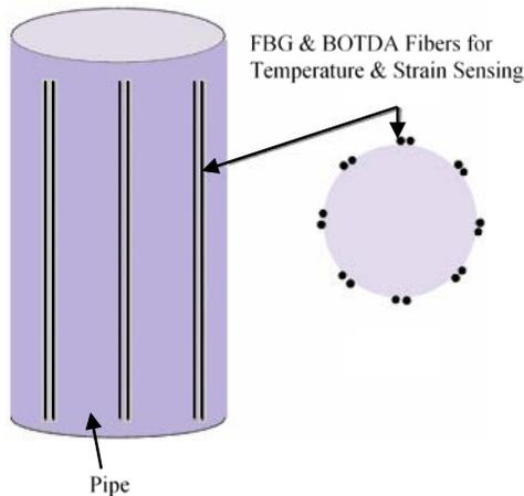
Figure 12. FBG and BOTDA fiber sensors attached along the longitudinal direction of the pipe for temperature and buckling detection (Revised from Leung et al., 2013)
