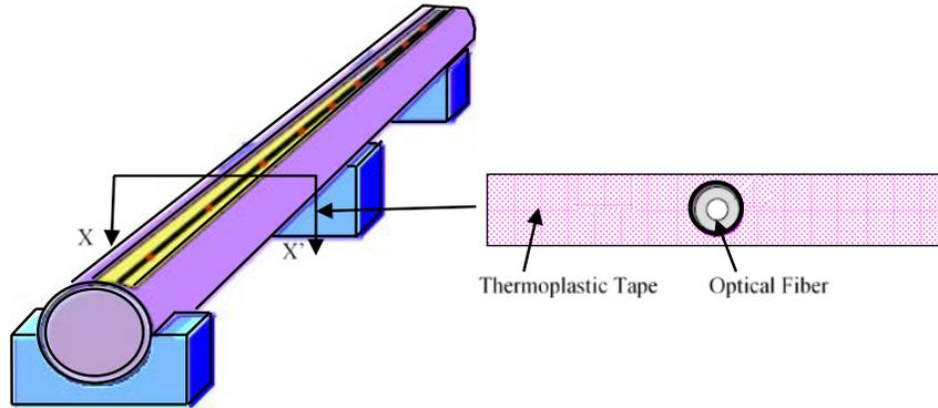
Figure 10. Cross- section and application of sensing tape (Revised from Inaudi and Glisic, 2007)
