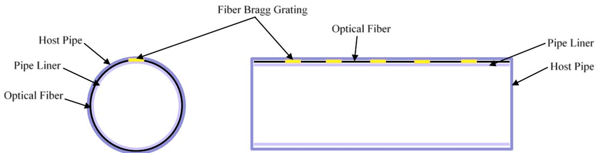
Figure 13. Schematics of FBG Sensors installed in pipe liner (Revised from Saber and Sterling, 2005)
