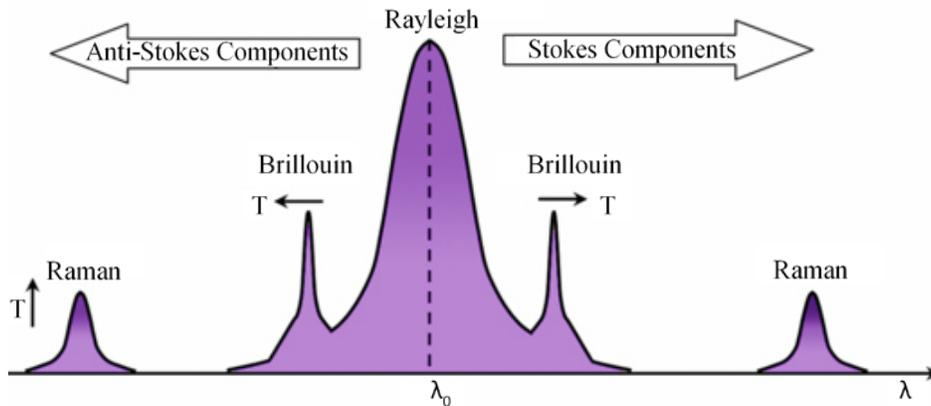
Figure 3. Optical scattering components in optical fibers. (Revised from Zhou et al., 2012)
