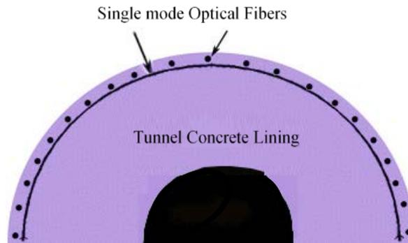
Figure 7. Application of FOS for monitoring a tunnel concrete lining (Revised from Leung, et al., 2013)
