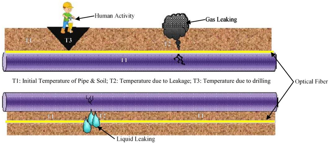
Figure 11. Detection of gas/liquid leak through a cable placed on/under the pipeline (Revised from Inaudi and Glisic, 2007)
