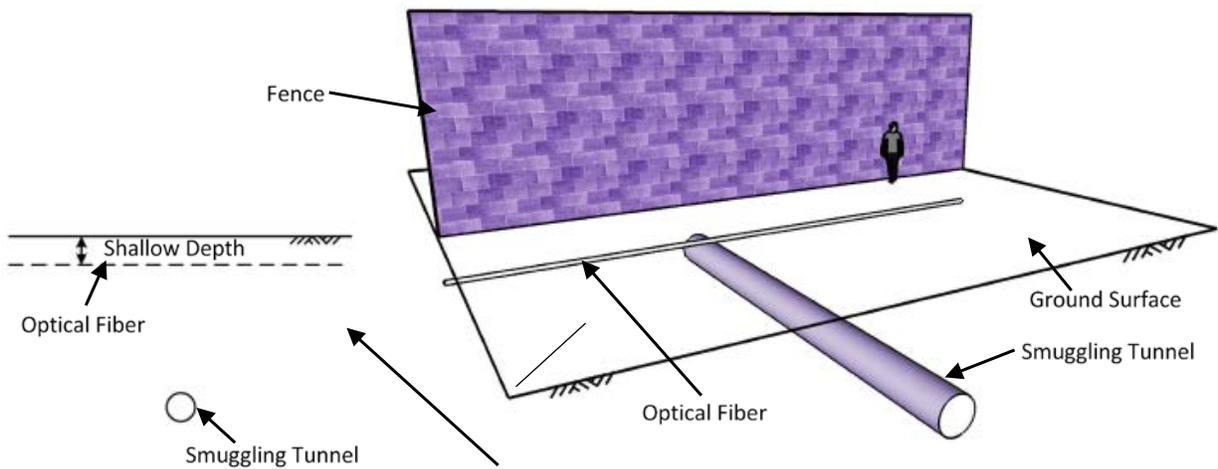
Figure 9. Detection of smuggling tunnel using FOS (Revised from Linker and Klar, 2013)
