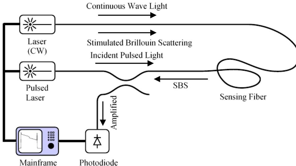
Figure 4. Working principle of OTDR (Revised from Schenato, 2017).
