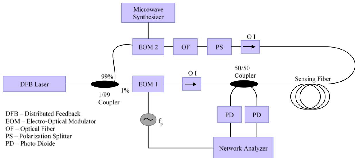
Figure 5. Working principle of BOFDA (Revised from Bernini et al., 2005)
