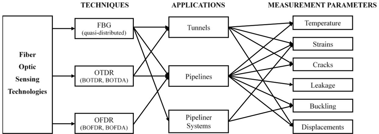
Figure 6. Overview of monitoring applications of underground infrastructure using fiber optic sensing technologies
