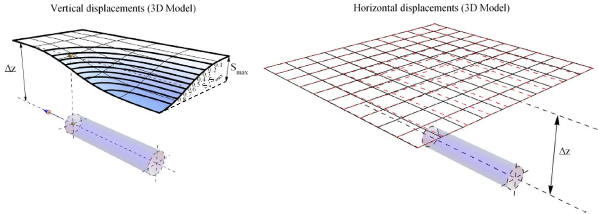
Figure 8. Illustration of vertical and horizontal ground displacements (Revised from Klar et al., 2014)
