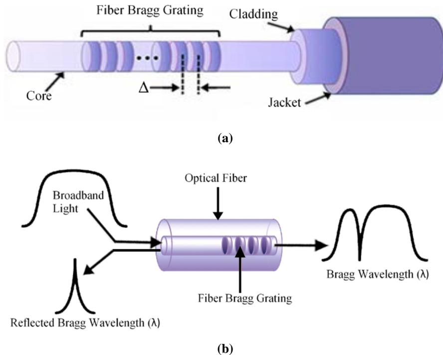
Figure 2. (a) A typical cross section of FBG sensor and (b) illustration of its working fundamental principle of FBG Sensor (Revised from National Instruments, 2016).
