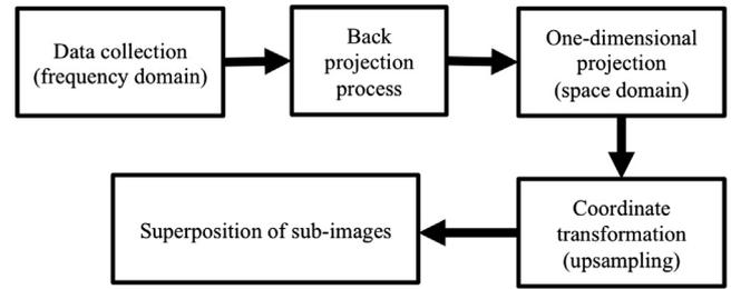
Fig. 2. Backprojection algorithm processing steps.
