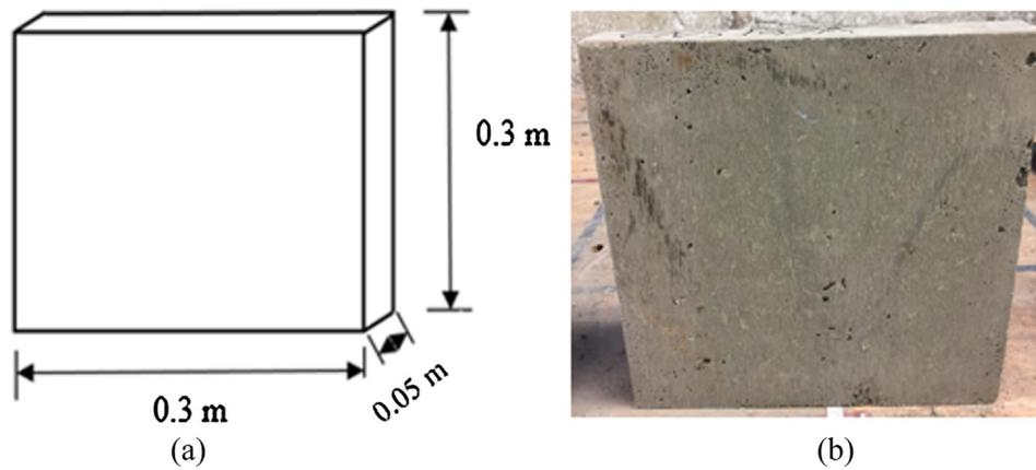
Fig. 3. Schematic (a) and picture (b) of concrete panel.
