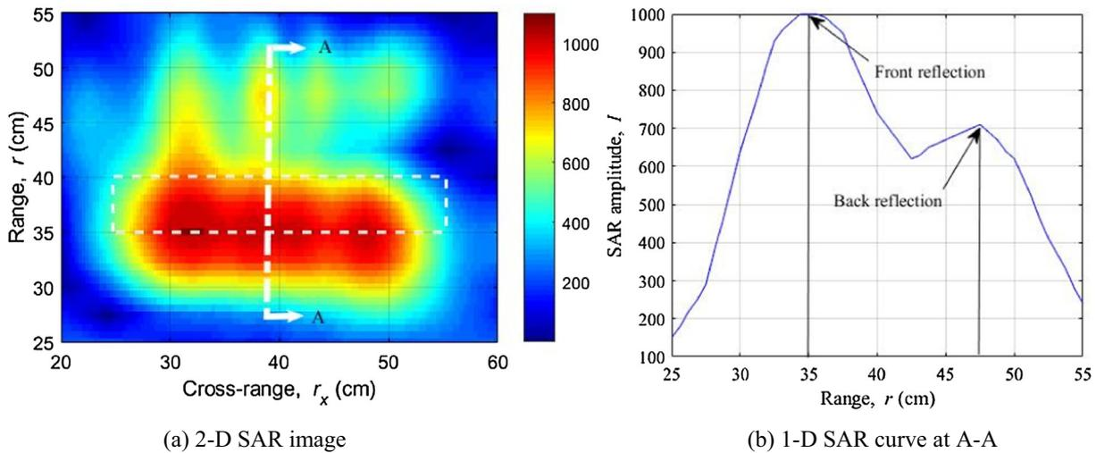
Fig. 8. 2-D SAR image and 1-D SAR curve of concrete at  $\psi = 0\%$ .
