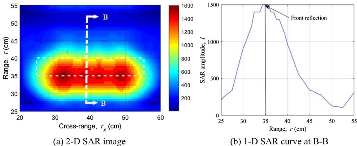
Fig. 9. 2-D SAR image and 1-D SAR curve of concrete at  $\psi = 3.85\%$ .
