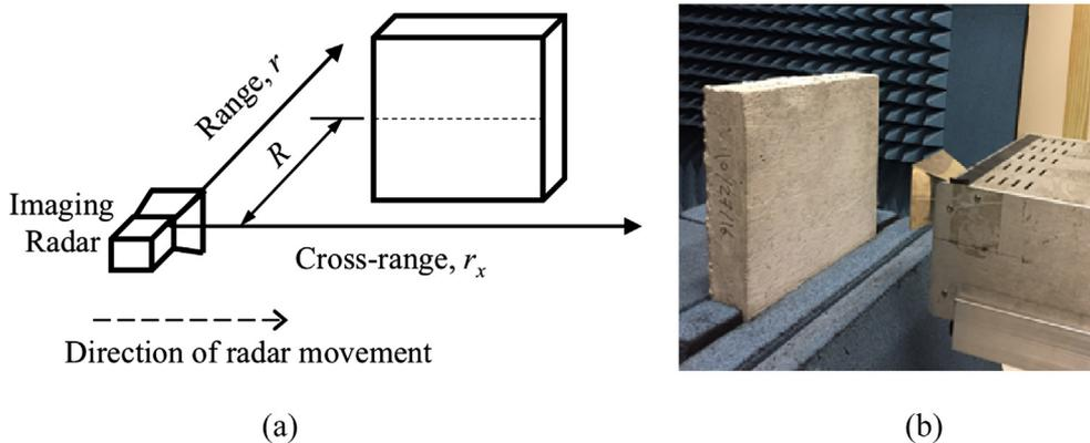
Fig. 4. Schematics (a) and picture (b) of SAR imaging system.
