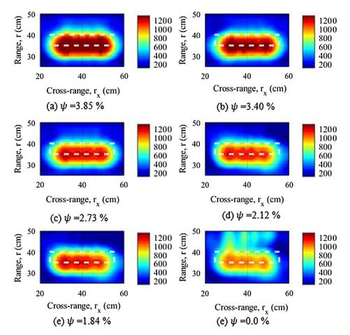
**Fig. 5.** SAR images of concrete panel at different moisture contents ( $\psi$  = moisture content).
