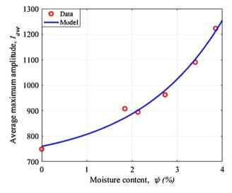
Fig. 7. Average maximum SAR amplitude vs. moisture content.
