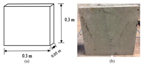
Fig. 3. Schematic (a) and picture (b) of concrete panel.
