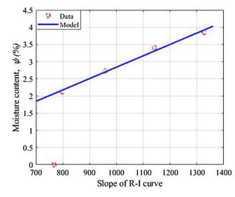
**Fig. 16.** Slopes of R-I curves representing different moisture contents ( $\psi = 0\%$ -3.85%).
