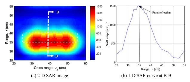
**Fig. 9.** 2-D SAR image and 1-D SAR curve of concrete at  $\psi$  = 3.85%.
