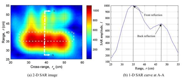
Fig. 8. 2-D SAR image and 1-D SAR curve of concrete at  $\psi$  = 0%.
