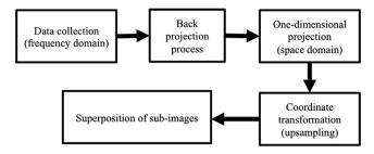
Fig. 2. Backprojection algorithm processing steps.
