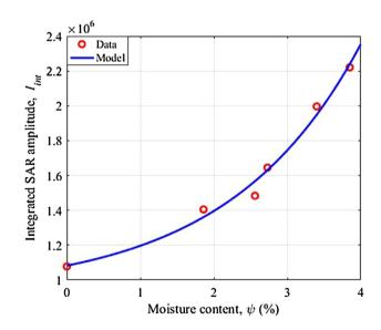
Fig. 6. Integrated SAR amplitude vs. moisture content.
