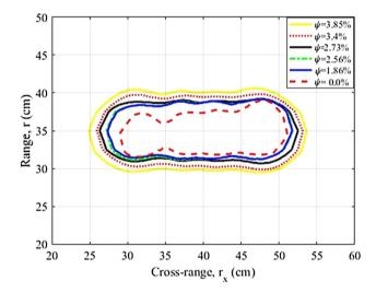
**Fig. 12.** Critical contours from SAR images representing different moisture contents (at *I* = 900).
