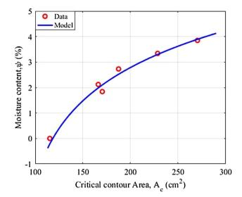
Fig. 11. Moisture content estimation by using critical area contour (at *I* = 900).
