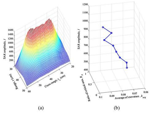
**Fig. 13.** K-R-I curve of a SAR image of concrete – moisture content  $\psi$  = 3.85%.
