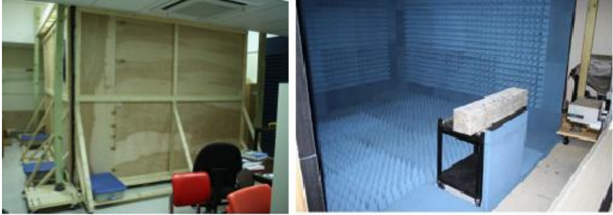
Figure 5. Custom-built anechoic chamber, 1 GHz-18 GHz; (left) exterior of the chamber, (right) interior of the chamber with a reinforced concrete beam specimen (CEE, UML)
